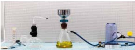
**The 'heart' of the lab is the test bench facility** which has been specially designed to validate the operating characteristics and performance of elements and filters. These advanced work stations offer pinpoint accuracy in measuring the level of contamination from solid particles in oils under pressure.
