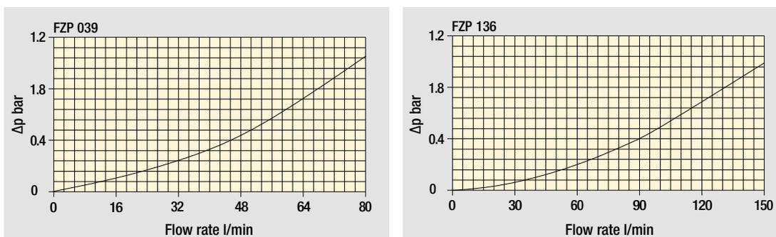
The curves are plotted using mineral oil with density of 0.86 kg/dm<sup>3</sup> in compliance with ISO 3968.  $\Delta p$  varies proportionally with density.
