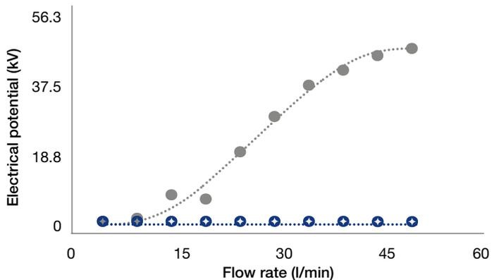
Under standard working conditions, the potential goes from tens of kV to zero, clearly showing the effectiveness of our dissipative filters.
