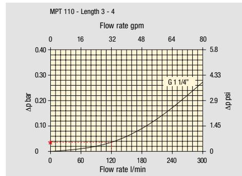
Filter housings  $\Delta p$  pressure drop. The curves are plotted using mineral oil with density of  $0.86 \text{ kg}/\text{dm}^3$  in compliance with ISO 3968.  $\Delta p$  varies proportionally with density.
