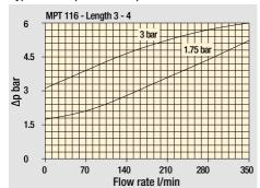
The curves are plotted using mineral oil with density of 0.86 kg/dm³ in compliance with ISO 3968. Δp varies proportionally with density.
