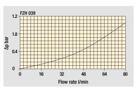
The curves are plotted using mineral oil with density of 0.86 kg/dm³ in compliance with ISO 3968.  $\Delta p$  varies proportionally with density.
