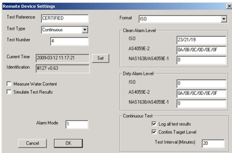
**Figure 2** Setting ISO Target Cleanliness Level
